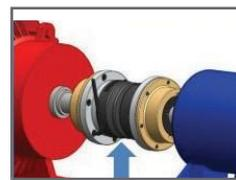
4. If necessary, use a sling to insert the TCAE in a horizontal position. Compressing and expanding the TCAE as necessary, slide it between both flanges. Secure the TCAE to both flanges by tightening the bolts in a diametrically opposite sequence.
