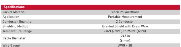
Capacitance 49 pF/ft (nom) conductor to shield
