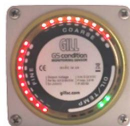
Red (Flashing) - Maximum debris condition breached
