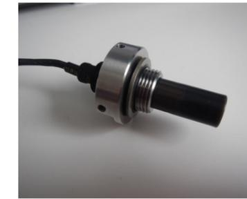
Sensor head with thread adaptor fitted
