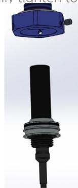
Carefully fit the Sensor Probe into the Thread Adaptor: There may be some resistance as the probe pushes past the internal o-ring seals. When the sensor is fully home it will hit a stop and the rear surfaces of the 2 parts will be at the same level. Secure the 2 parts together by tightening the grub screws using a 2mm hex key to a torque of 1Nm.
