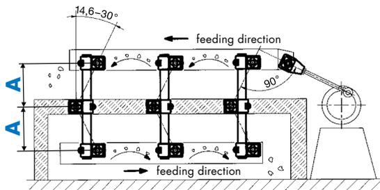
The three AR mounts are inserted on the round connecting tube, with the direction inverted center element. This so said "boomerang"-configuration is offering on the counter-mass trough a direction inverted flow of material, what could simplify selection and screening processing.
