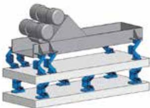
If, due to the demands of the process, large screens are mounted at a very high position in a building or in a purely steel construction, the transmission of the residual forces of a single-mass machine can set the
