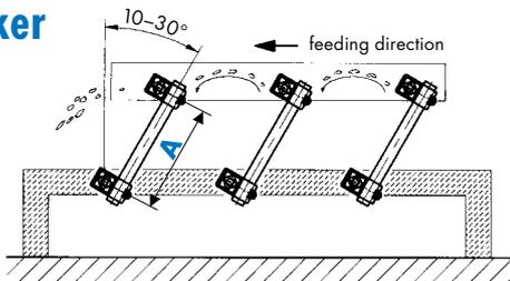
The two AR mounts are inserted on the round connecting tube. The required center distance should be positioned on the straightening plate (parallelism), subsequently tightening of the two collars with the required fastening torque.
