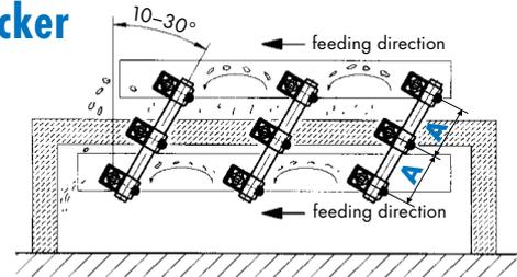
The three AR mountings are inserted on the round connecting tube (please check required material thickness by the relevant center distance on below-mentioned table). The counter-mass can be used as second trough with identical feeding direction.
