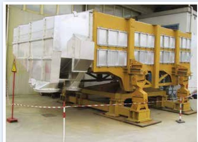
Wood-chip sorting screen mounted on 8 pcs. AK 100-4 suspensions
