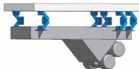
Discharge chutes under silos are normally supported by means of complicated yoke constructions and are suspended on pressure springs. With its HS suspensions (HS = hanging screen), ROSTA offers the possibility of the direct, cost-effective suspension of the discharge unit on silos and bunkers. The geometry of the HS suspensions has been designed to accommodate tensile loads.
