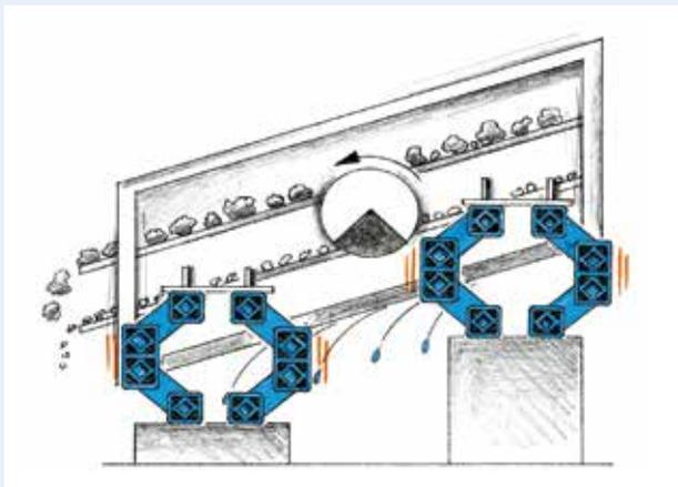
Circular motion screens or circular vibrators are normally excited by unbalanced weights that create a circular rotating oscillation of the screening frame. Relatively low accelerations of the screened material are achieved with this form of excitement. Circular vibrators thereby normally work with a screening frame inclination of  $15^\circ$  to  $30^\circ$ , so that an adequate material throughput is ensured.
