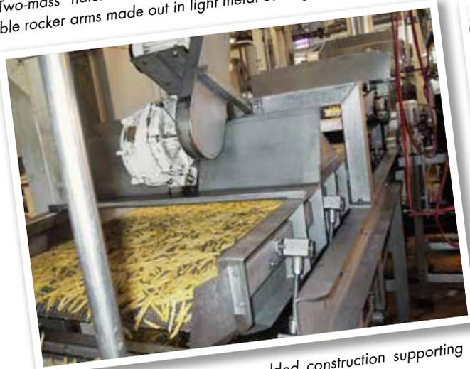
Stainless steel rocker arms in welded construction supporting a foodstuff shaker conveyor
