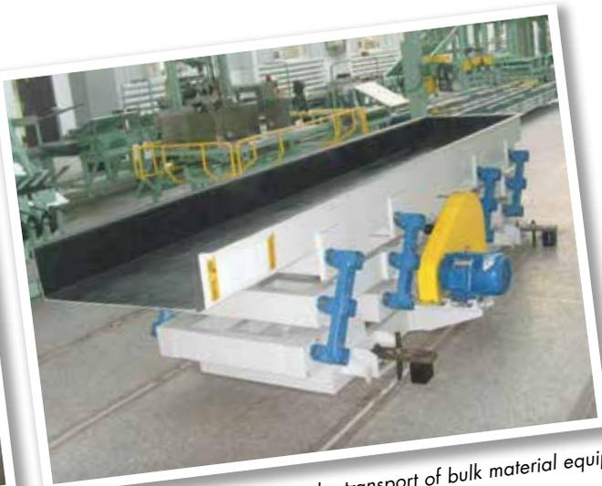
Two-mass shaker conveyor for the transport of bulk material equipped with double rocker arms AD-P 50
