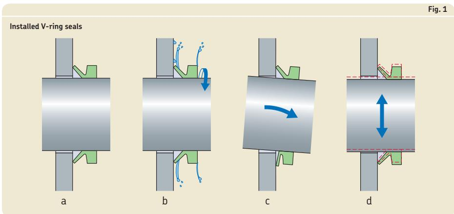
low but sufficient enough to maintain the sealing function. The light contact pressure even enables the seal to run dry in some low-speed applications resulting in insignificant torque drag or heat build-up. The contact pressure varies with the fitted width.
